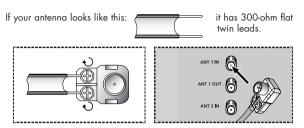
Place the wires from the twin leads under the screws on the 300-75 ohm adaptor (not supplied). Use a screwdriver to tighten the screws. Plug the adapter into the "ANT 1 IN" terminal on the rear panel.
